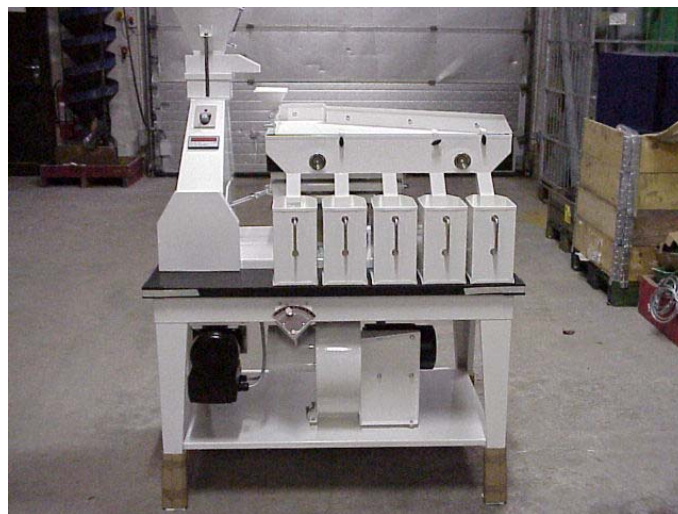
Figure 5.1: Laboratory scale gravity separator
